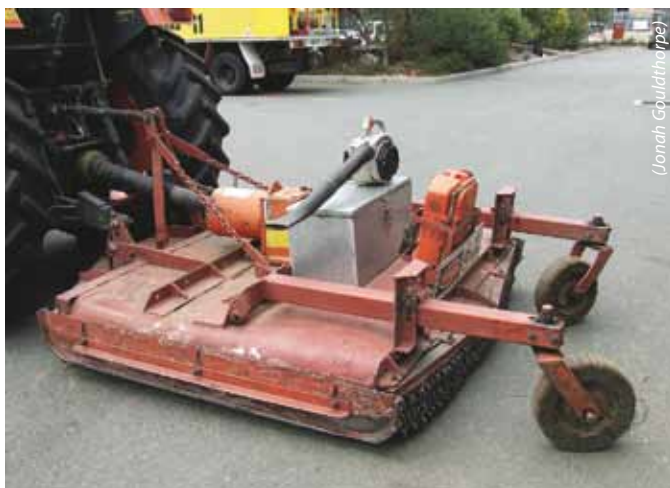
Machinery hygiene in the ACT. The blower is carried on the slasher deck for cleaning in the field
